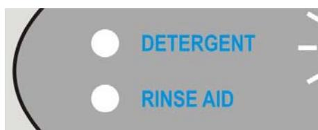
Detergent and Rinseaid is continuously monitored (by conductivity) on entry into the machine.
